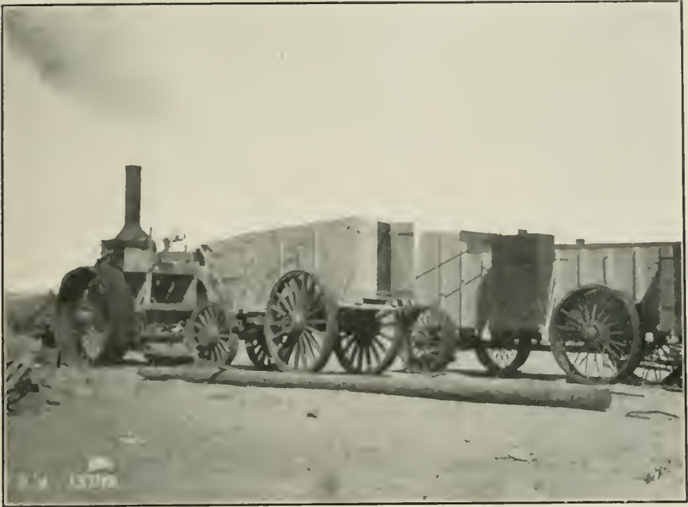
DESERT WAGONS—LOCOMOBILE TRAINS USED AT DANBY SALT MINES ON MOJAVE DESERT, SAN BERNARDINO COUNTY.
